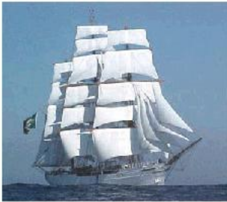
The Sullivan's Pier - Staten Island 3 masts - 32 sails - 250 ft long Full Rigged, built 1982
