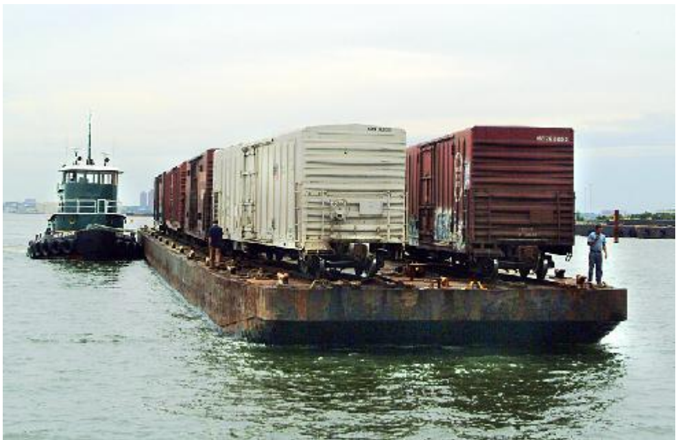
An image of a car float (carrying RR cars) being towed "on the hip" by a tug Note the lookout crew member on the barge with radio - the captain can't see! Photo (c) Bernard Ente
